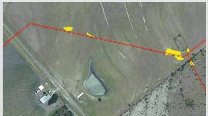
Figure 1. Example of Satelytics leak detection.
